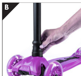
Pull the fixing sleeve upward, as shown in Figure B and Figure C
