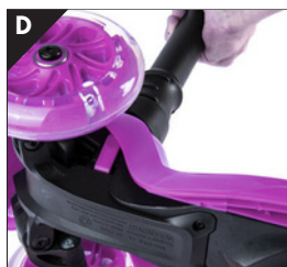
Press Red Push Switch with one hand and using the other hand to pull handlebar to separate the handlebar and scooter body, as shown in Figure D and Figure E.
